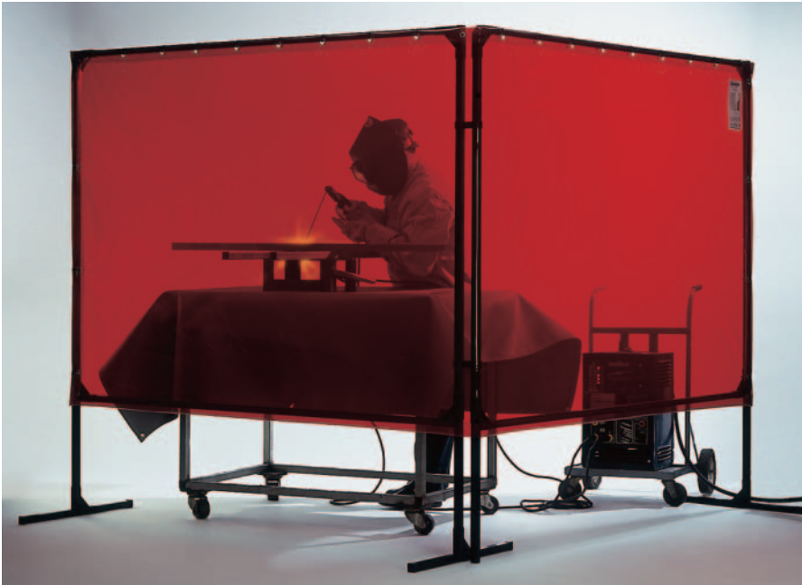
Fig. 2 — Transparent welding curtains can be designed to interlock to completely enclose a work area. The ideal TWC allows those passing by to safely view the interior of the booth in detail.
